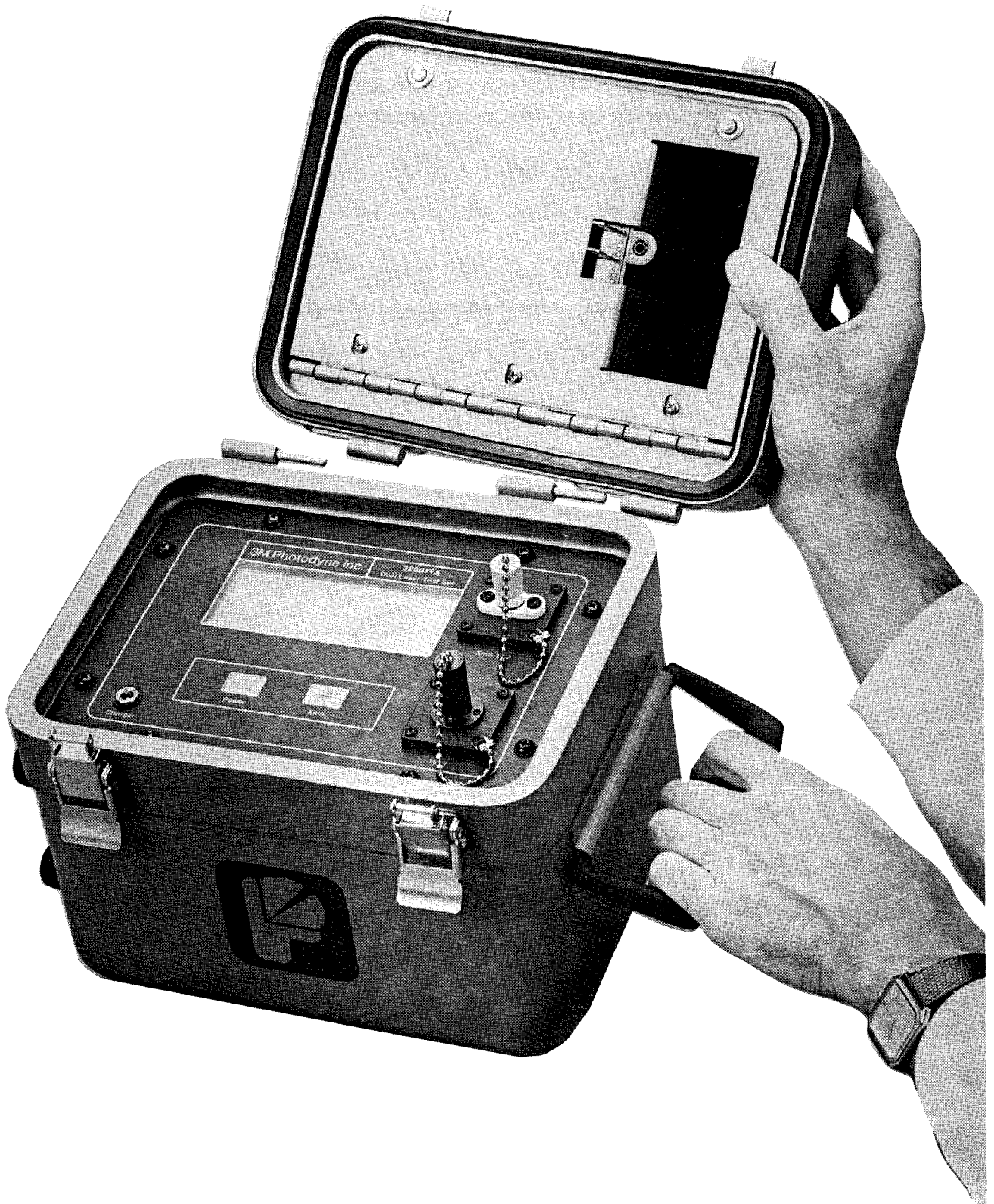
Figure 9.1 Removing Top Cover of Test Set
